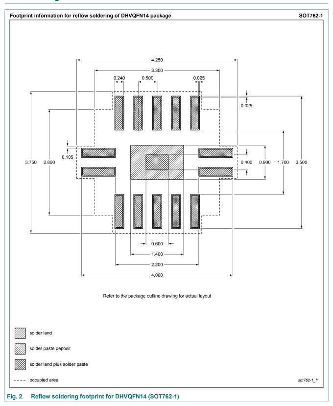
plastic, leadless dual in-line compatible thermal enhanced very thin quad flat package; 14 terminals; 0.5 mm pitch; 2.5 mm x 3 mm x 0.85 mm body
